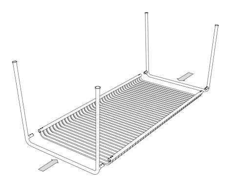
Firmly secure the legs by fastening the screws with the supplied Allen key.
