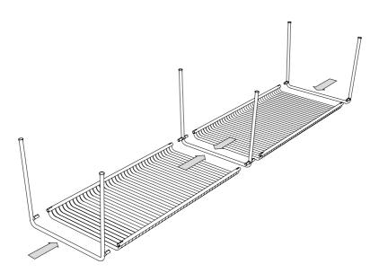
Firmly secure the legs by fastening the screws with the supplied Allen key.
