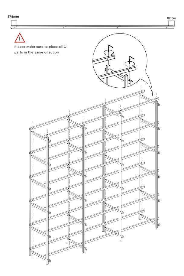
Place the screw to connect the A part and C part. Tighten the screw gently. When all screws are placed and fully tightened, place the F part on the screw heads.
