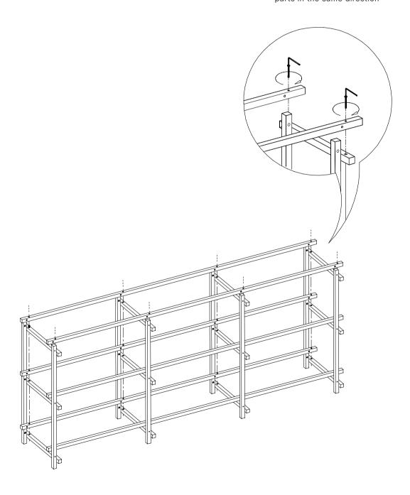
Place the screw to connect the A part and C part. Tighten the screw gently. When all screws are placed and fully tightened, place the F part on the screw heads.
