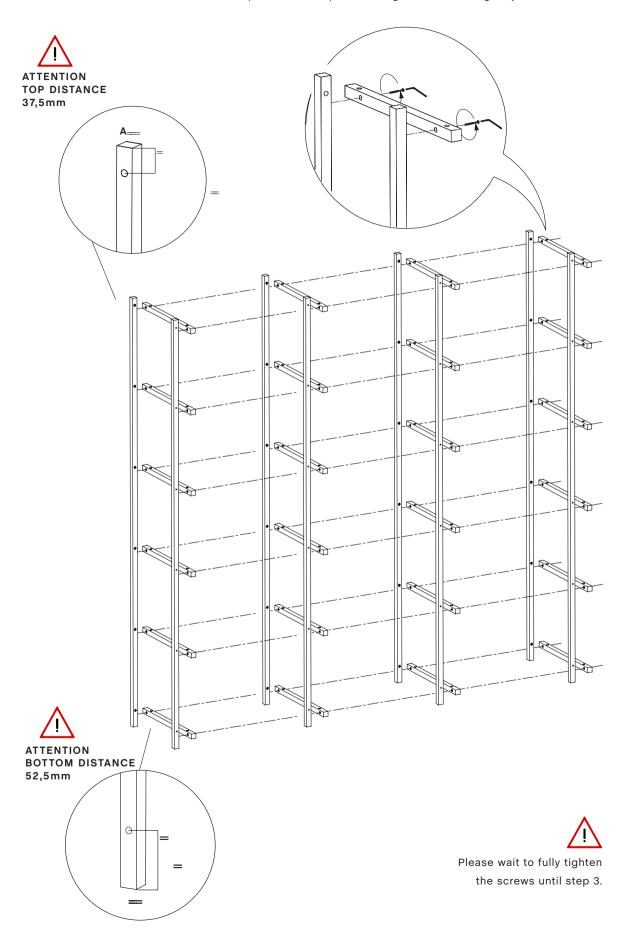
Place the 12 x C parts and gently tighten the screw. 2 persons are recommended to complete the following steps
