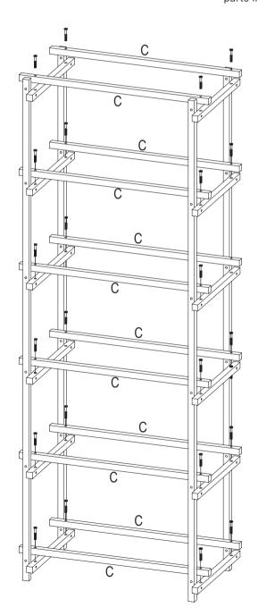
Place the screw to connect the A part and C part. Tighten the screw gently. When all screws are placed and fully tightened, place the F on the screw heads.
