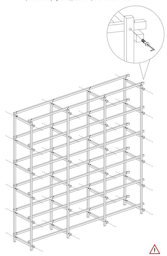
Please make sure to tighten all screws fully before placing the F part.
