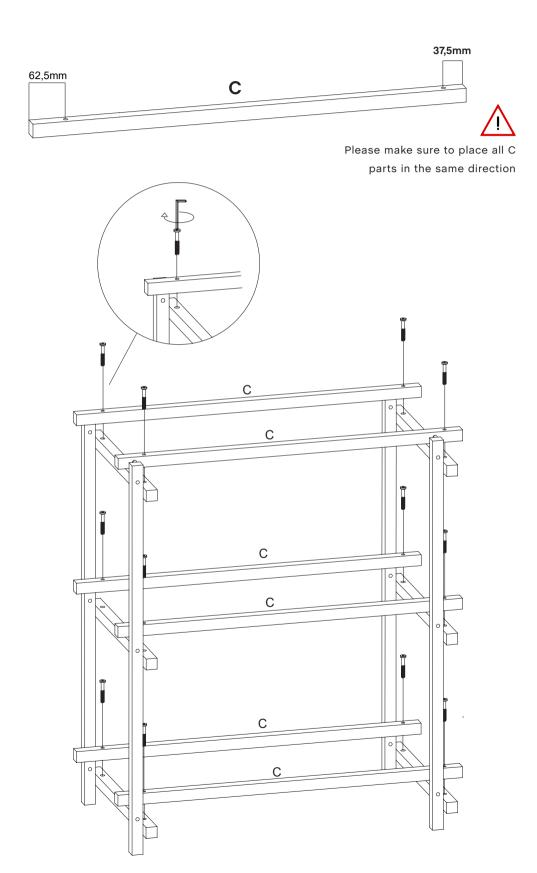
Place the screws to connect the A part and C part. Tighten the screw gently. When all screws are placed and fully tightened, place the F on the screw heads.
