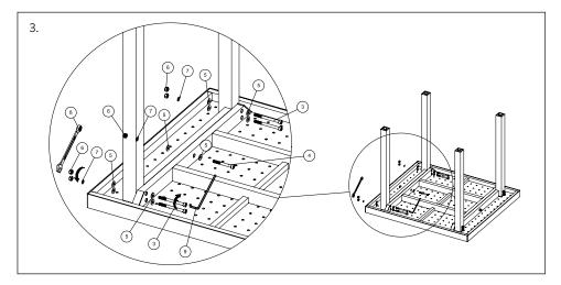
3. Attach all bolts, nuts and discs loosely. Once they are in place, tighten.
